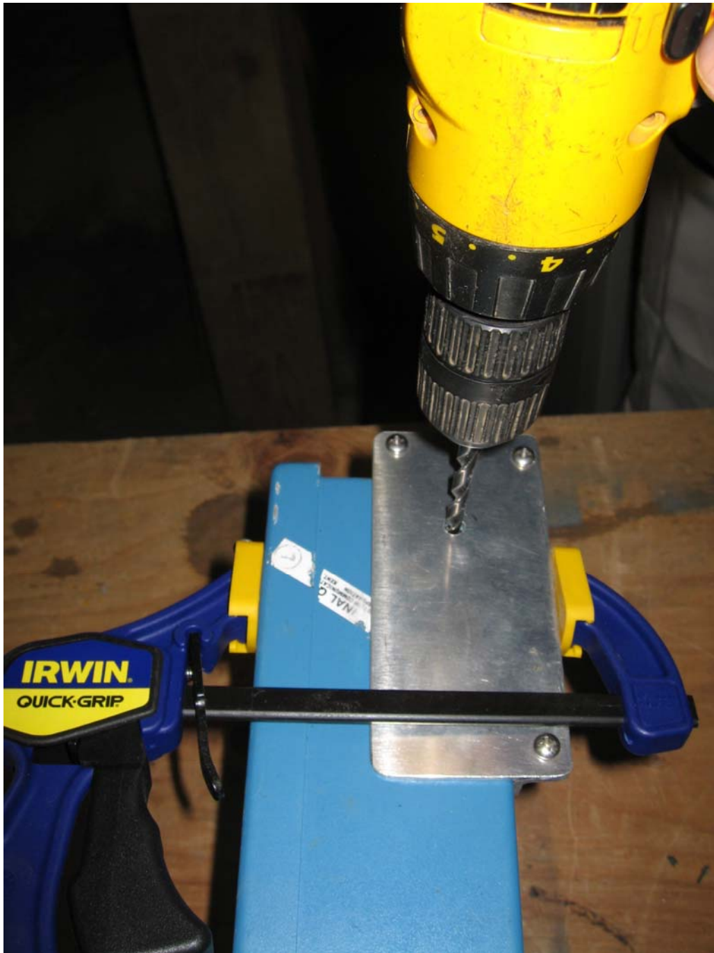
Figure One – Drilling the Pin Latch Hole
