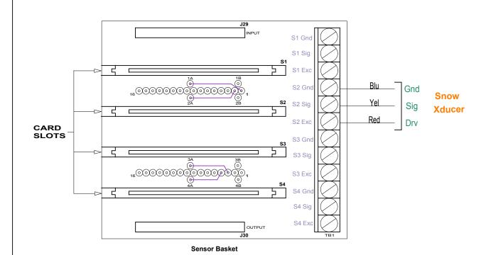
Violet lines are wires that program each sensor card's position in the data stream
